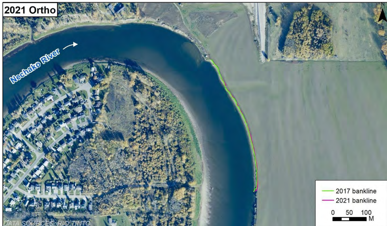
Figure 4.27 Comparison of 2017 and 2021 bankline positions along the agricultural field located near RKM 156.
