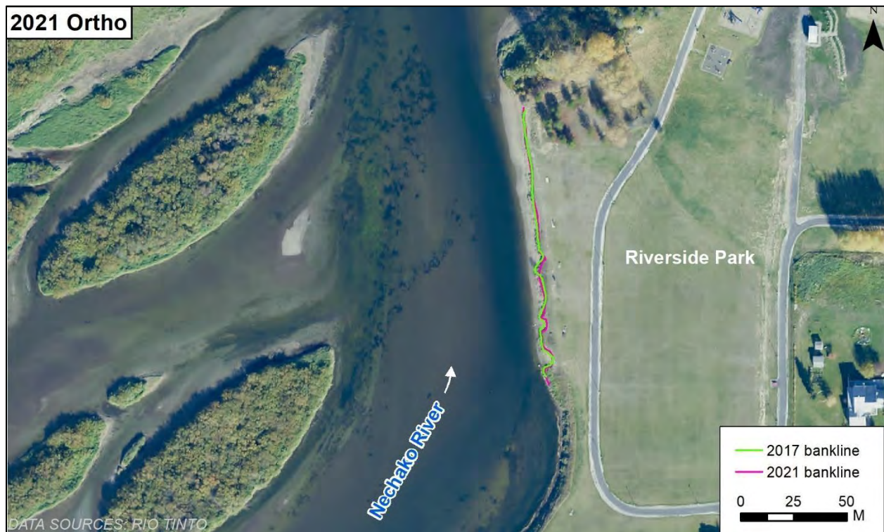
Figure 4.26 Comparison of 2017 and 2021 bankline positions at Riverside Park located at RKM 152.5.
