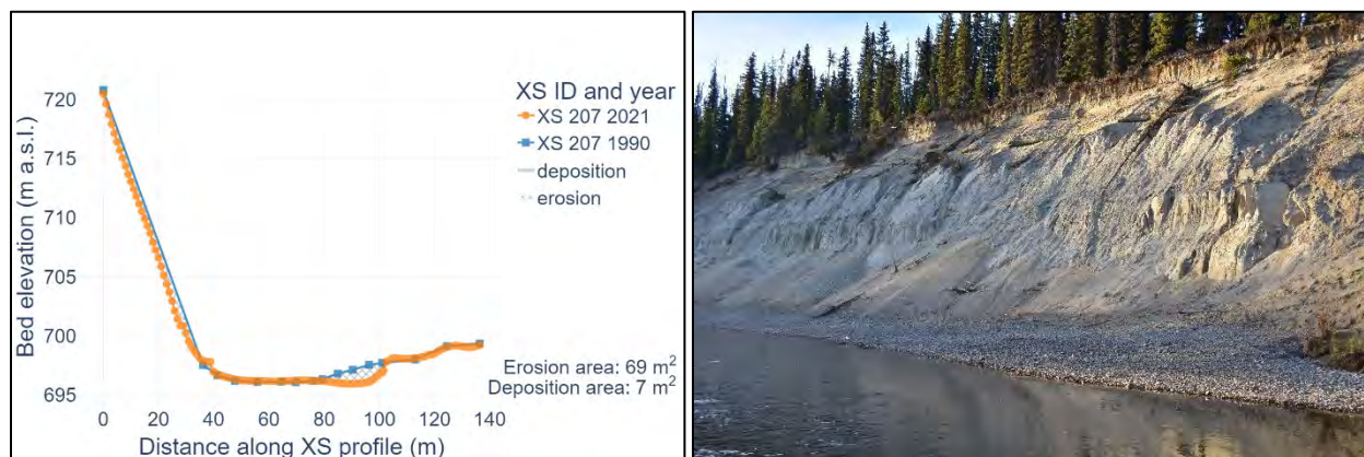
Figure 4.11 Minor erosion of the high cutbank at XS 207 (1990-2021).
